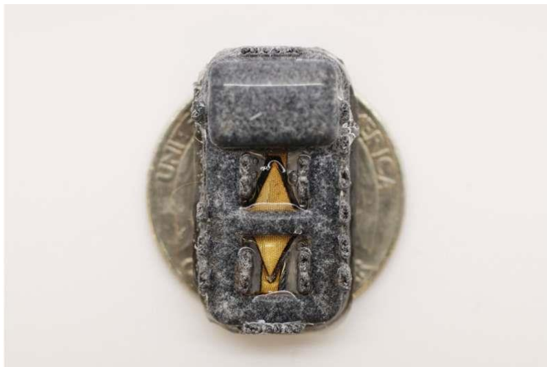
Optical image of cathode side of fully assembled O 2 -Macrodevice showing, with a United States quarter-dollar coin for scale. Credit: Claudia Liu and Dr. Siddharth Krishnan, MIT/Boston Children's Hospital
